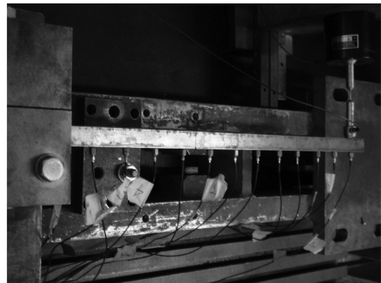
Fig. 6 Experimental setup showing the accelerometers and the shaker applied to the surface of the beam opposite to accelerometer 13; the larger saw cut (case B) is visible after accelerometer 5.
